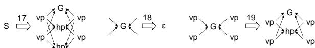
Figure 3: Extra production rules for 3D cabinets. Note that these extra rules are in the same grammar as the one in Figure 2. vp represents a vertical-panel part, h represents a horizontal-panel part, and G is for adding more horizontal-panel parts.
