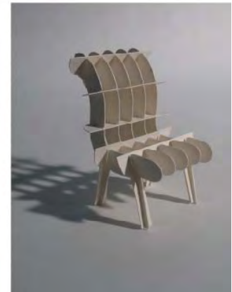
Figure 10. Paper chairs created using the system and cut with a cutter plotter (each chair is about 70 mm in height).
