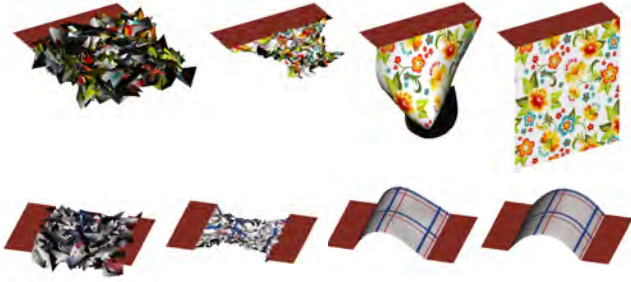
Figure 6: Stability Benchmark: (top) Snapshots at initial, third, 50th, and 200th iterations for the draping of a rectangular (membrane-dominated) textile (3K triangles, 12s total computation). (bottom) Snapshots at initial, third, 50th, and 100th iterations for static equilibrium of a rectangular (bending-dominated) thin plate with bending stiffness 100\times that of textile (2K triangles, 4s total computation).
